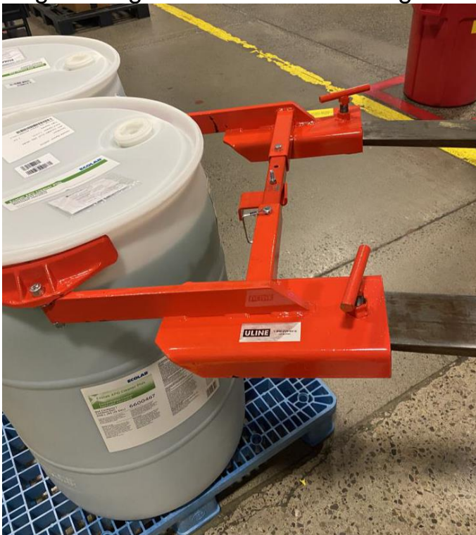
Engineering control #3: Drum lifting aid attachment to existing fork lifts
