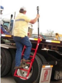
Worker using a “Deckmate” ladder to climb on trailer
