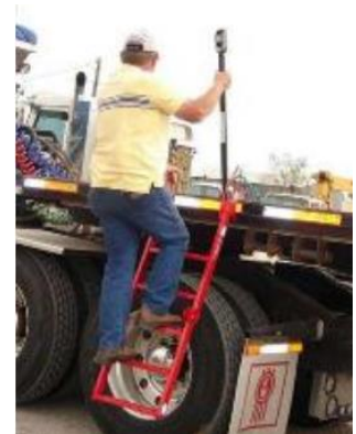
Getting on flatbed trailer using a flatbed ladder
