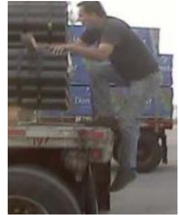
Getting on flatbed trailer using the rub rail and bumper for support
