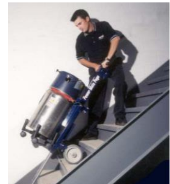
Transporting equipment up stairs using a stair climbing hand truck
