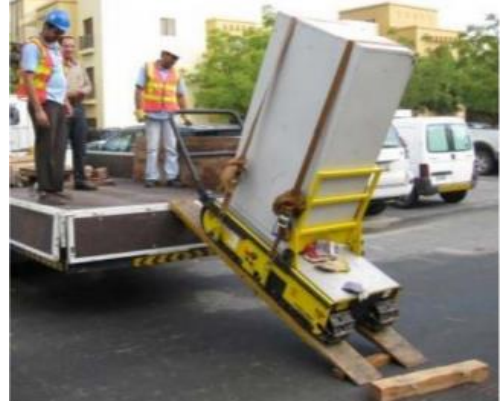
Transporting equipment up stairs using a stair climbing hand truck
