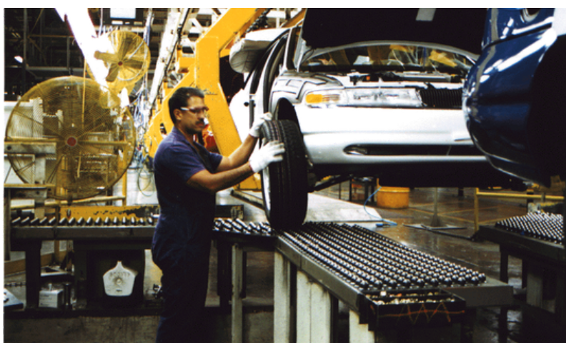
A worker completing the wheel decking job using the improved roller table to align the wheel in the wheel well.
