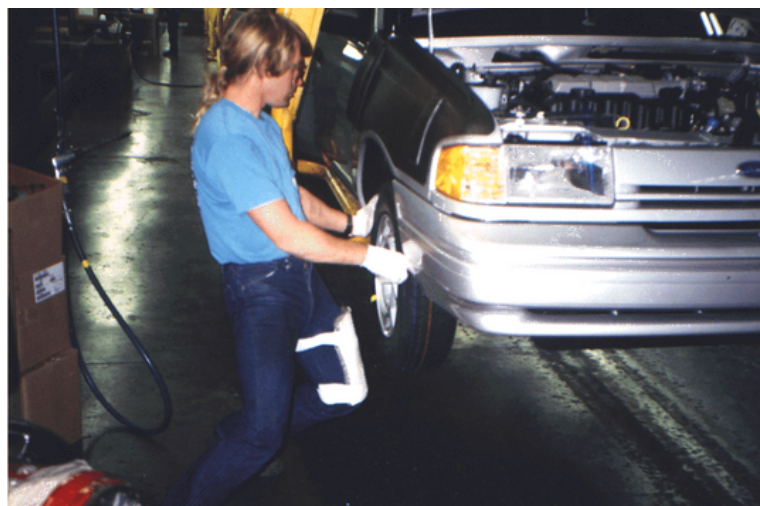
Worker completing the wheel decking task: manually lifting the wheel into the wheel well with the support of their knee. The worker added the knee pad due to previous injury from contact stress and discomfort.
